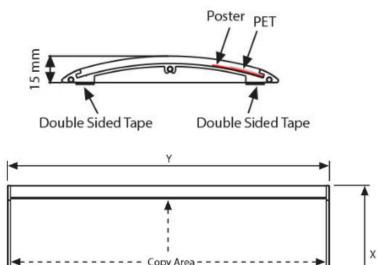
All curved aluminium signs in this range are supplied with black plastic end caps and come with a suction tool to make it easy to remove the plastic cover sheet.
