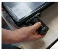
2. Screw springs onto base of frame.
