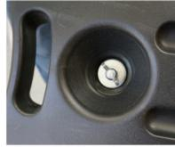
Insert bolt with washer into base undersi screw into springs and tighten.
