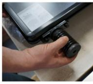
2. Screw springs onto base of frame.
