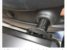
3. Place springs into locating holes on top of base.
