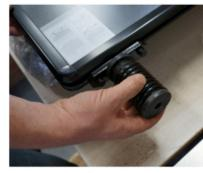
2. Screw springs onto base of frame.
