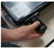
2. Screw springs onto base of frame.
