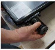
2. Screw springs onto base of frame.
