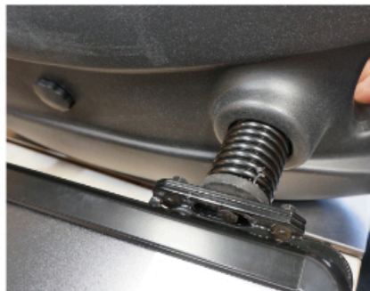
3. Place springs into locating holes on top of base.
