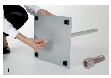
Identify the leg with two threaded screw ports inside. Using the two socket head bolts and the larger allen key connect the square base to the bottom leg and tighten up.
