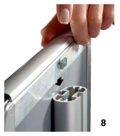
Open the snap frame. Choose portrait or landscape. Loosely assemble two mounting screws with lugs on the back to align with the channel in the leg.
